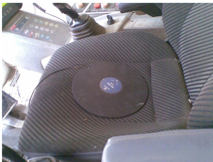
Figure 1: Position of vibrometer sensors on the seat
